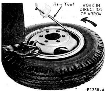
FIG. 9—Removing Slide Ring
