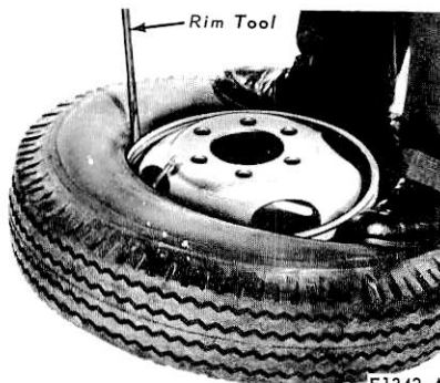
FIG. 13—Installing Tire Second Bead on Wheel
