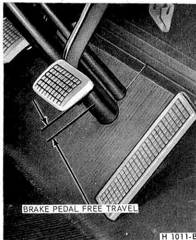
FIG. 1—Pedal Free Travel Check
