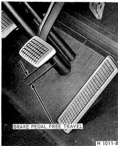
FIG. 1—Pedal Free Travel Check
