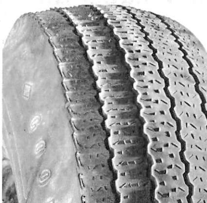
FEATHERING DUE TO MISALIGNMENT OR SEVERE CORNERING
