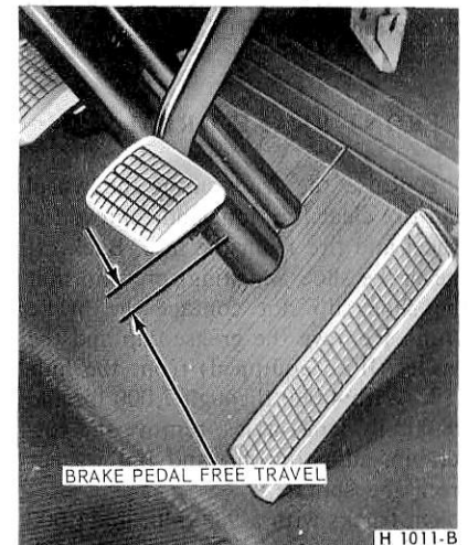
FIG. 1—Pedal Free Travel Check
