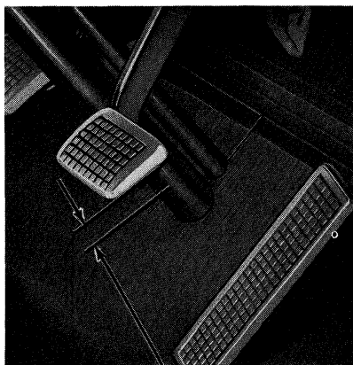
FIG. 1—Pedal Free Travel Check
