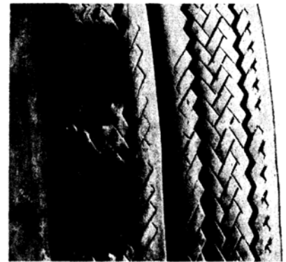
CUPPING—UNDERINFLATION AND/OR MECHANICAL IRREGULARITIES
