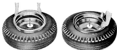
FIG. 4 Positioning and Starting Ring—Two-Piece Rim
