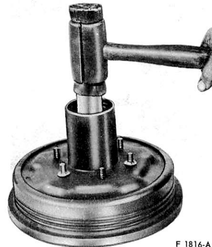
FIG. 26 Inner Bearing Cone and Grease Seal Removal
