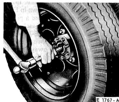
FIG. 5 Axle Shaft Removal—Tapered Dowels
