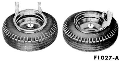
FIG. 4 Positioning and Starting Ring—Two-Piece Rim
