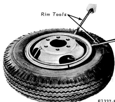
FIG. 7 Loosening Tire Bead
