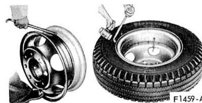
FIG. 2 Removing Ring and Loosening Tire Bead—Two-Piece Rim
