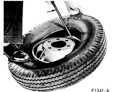
FIG. 10 Installing Tire First Bead on Wheel
