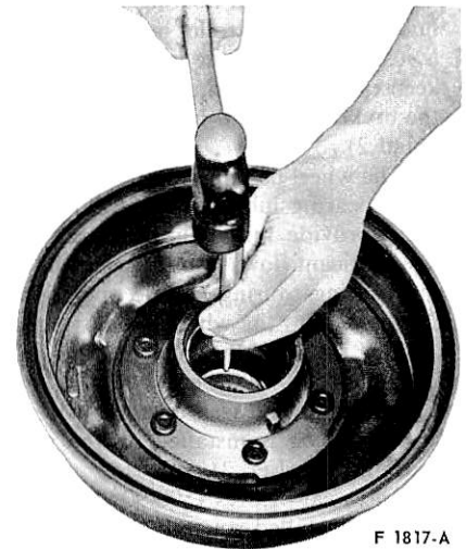
FIG. 27 Bearing Cup Removal
