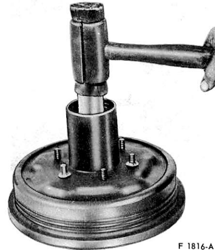
FIG. 26 Inner Bearing Cone and Grease Seal Removal
