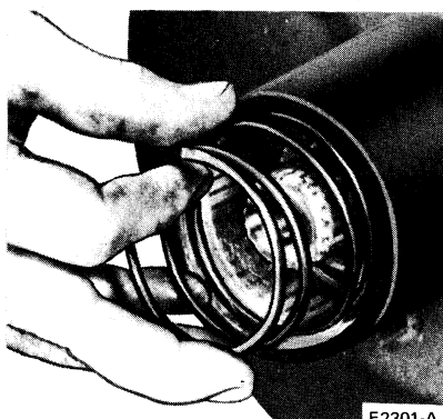
FIG. 9 Coil Spring Installation
