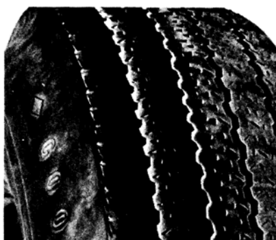
FEATHERING DUE TO MISALIGNMENT OR SEVERE CORNERING
