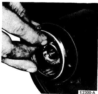
FIG. 8 Spring Retainer Ring Installation
