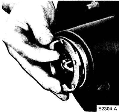
FIG. 12 Installing Cam Body Ring into the Clutch Retaining Ring
