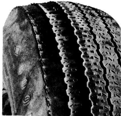
FEATHERING DUE TO MISALIGNMENT OR SEVERE CORNERING
