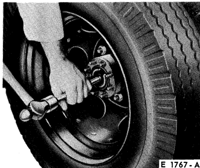
FIG. 5 Axle Shaft Removal—Tapered Dowels
