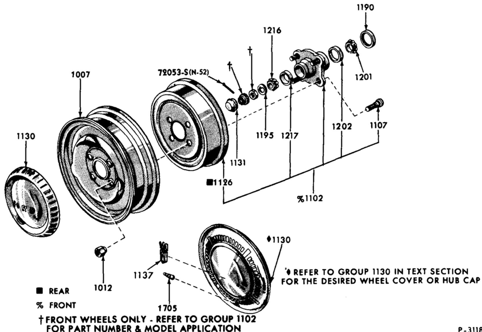
FRONT & REAR WHEEL, HUB, & BEARINGS - TYPICAL
