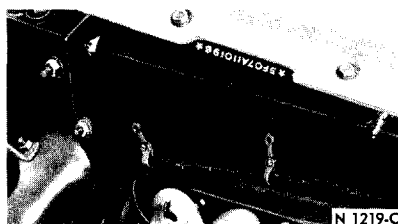
FIG. 5—Vehicle Identification Number Location—Comet, Falcon and Mustang
