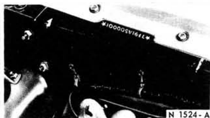
FIG. 3—Cougar Identification Number Location
