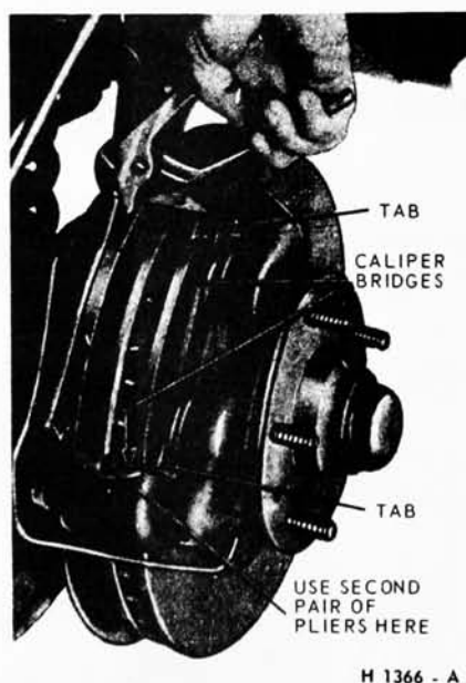
FIG. 7—Removing Disc Brake Shoe and Lining Assembly
