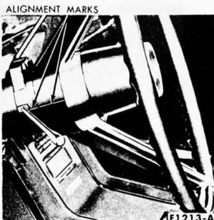
FIG. 3—Typical Straight Ahead Position Marks
