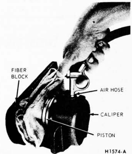
Fig. 10—Removing Piston from Caliper
