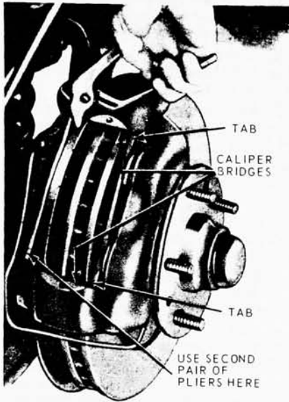
FIG. 9—Removing Disc Brake Shoe and Lining Assembly
