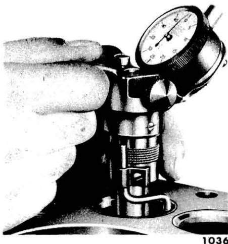
Fig. 12—Checking Valve Seat Runout
