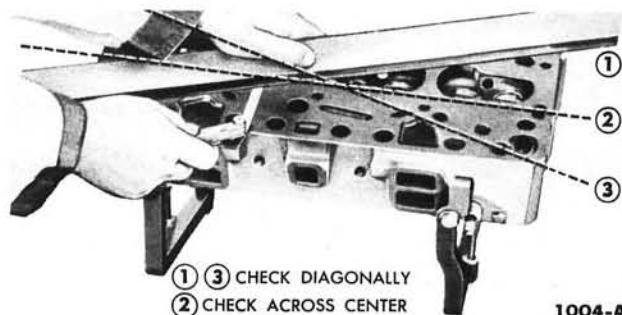
FIG. 4—Cylinder Head Flatness—Typical
