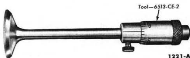
FIG. 23—Measuring Valve To Cap Clearance—Free Turning Valve
