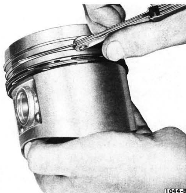
FIG. 64—Ring Side Clearance—Typical
