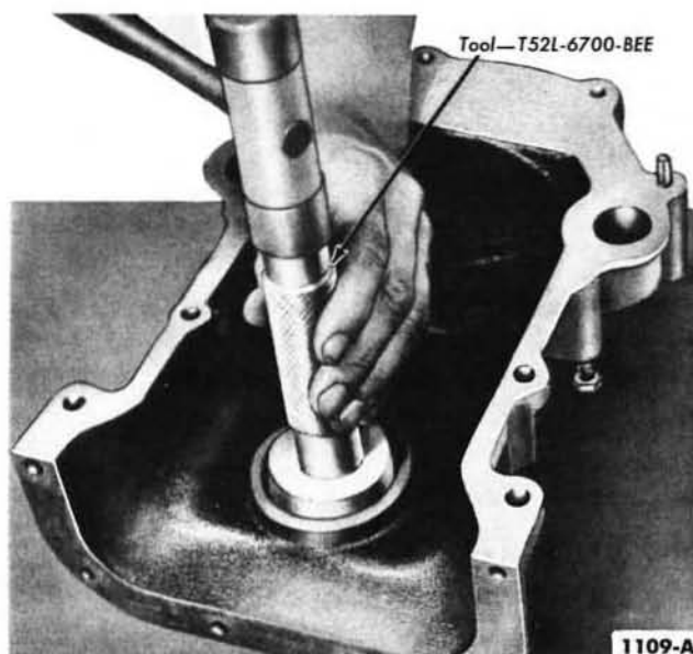
FIG. 41—Oil Seal Installation
