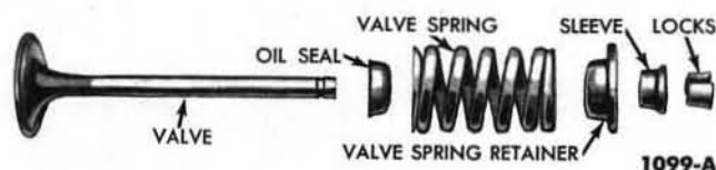
FIG. 24—Rotating Type Valve Assembly
