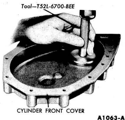
FIG. 36—Front Seal Installation
