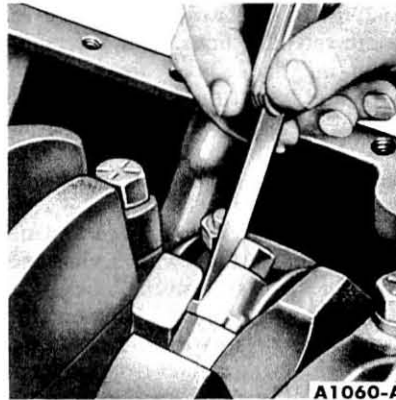
FIG. 33—Checking Side Clearance
