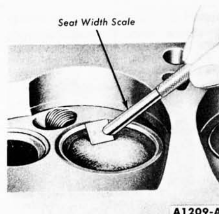
FIG. 7—Valve Seat Width
