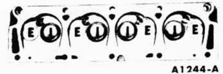
FIG. 6—Valve Port Arrangement
