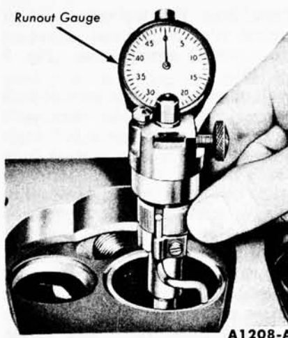
FIG. 6—Valve Seat Runout
