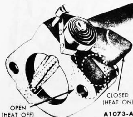
FIG. 4—Exhaust Gas Control Valve
