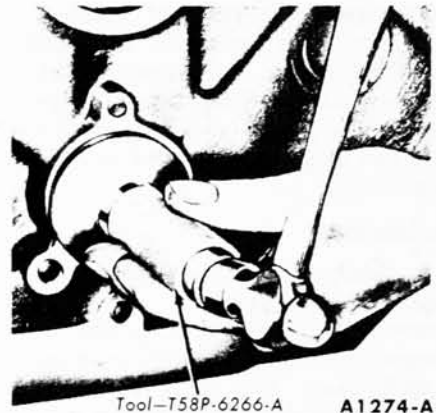
FIG. 33—Camshaft Rear Bearing Bore Plug Installation
