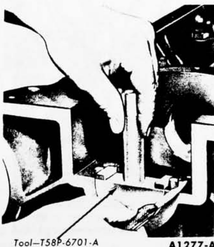
FIG. 36—Seal to Block Installation
