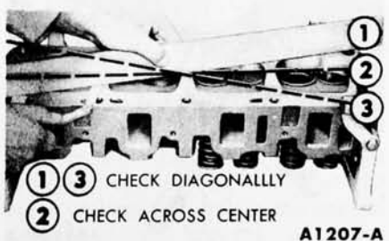
FIG. 5—Cylinder Head Flatness
