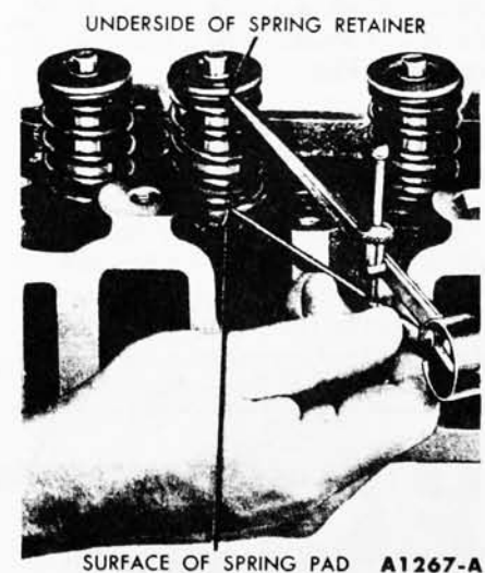
FIG. 26—Valve Spring Assembled Height
