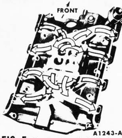
FIG. 5—Intake Manifold Fuel Passages
