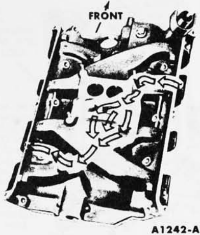
FIG. 3—Intake Manifold Exhaust Gas Passages
