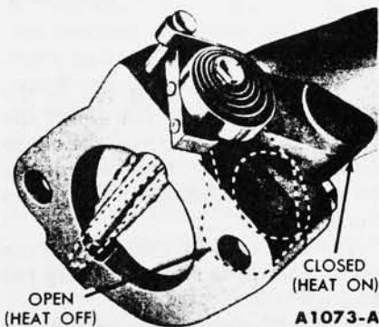
FIG. 4—Exhaust Gas Control Valve
