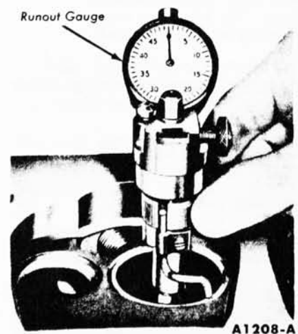
FIG. 38—Valve Seat Runout
