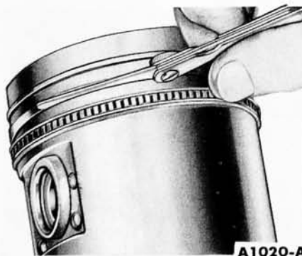
FIG. 69—Ring Side Clearance
