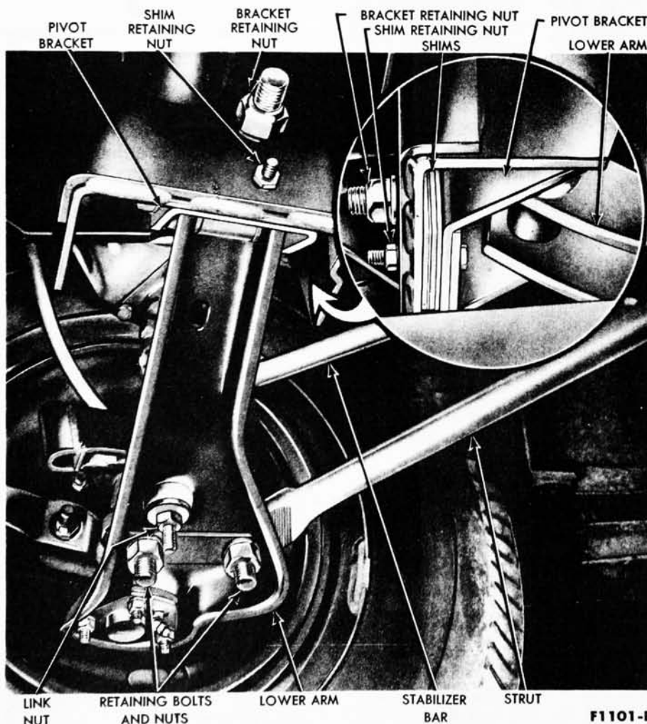
FIG. 9—Suspension Lower Arm Installed
