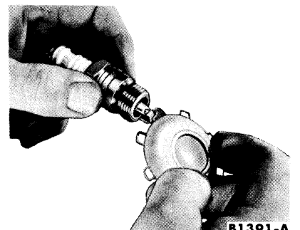
FIG. 2—Gapping Spark Plug
